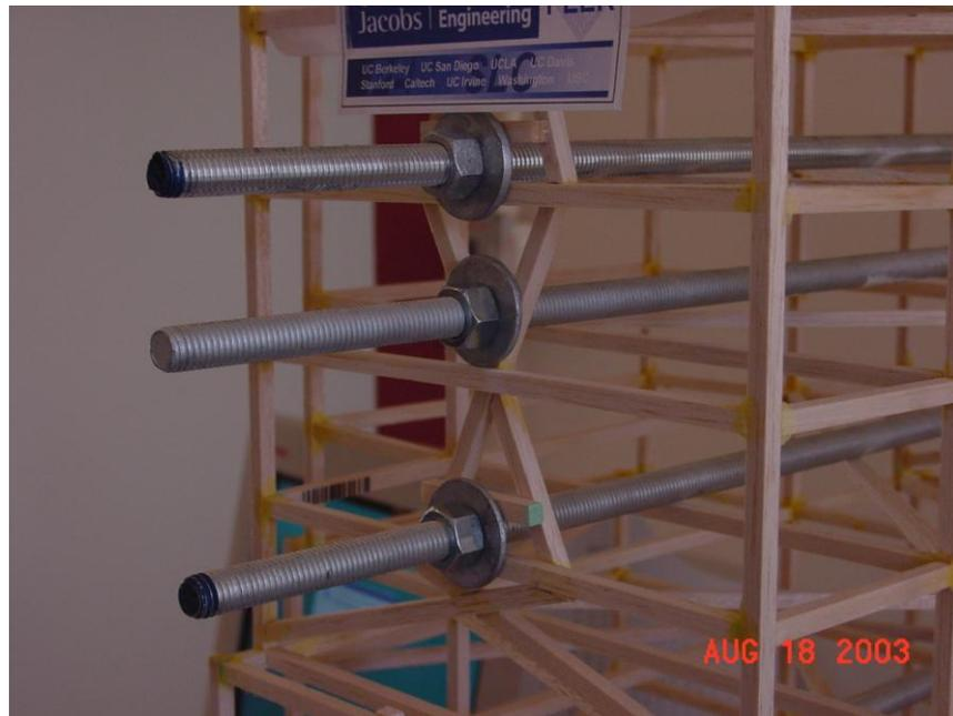
(a.) Example of insufficient support for threaded bars preventing the requisite tightening of the nuts, thereby permitting the bars to slide with respect to the structure during shaking. (The photo was taken at the 2003 competition, when weight distribution different from this year's configuration)
