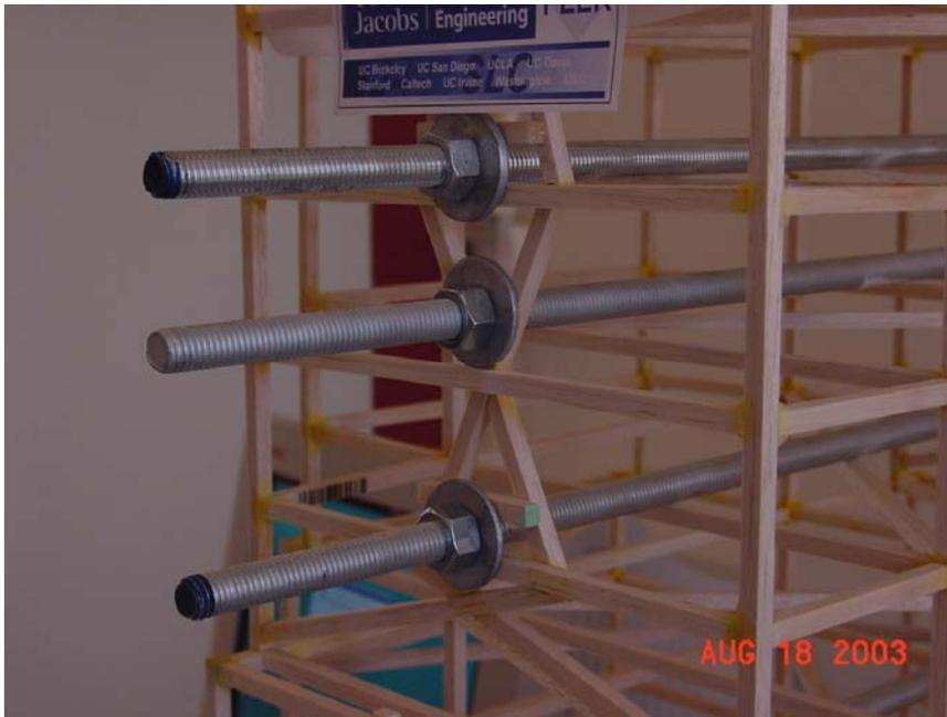
(a.) Example of insufficient support for threaded bars that prevent the requisite tightening of the nuts, thereby permitting the bars to move relative to the structure during shaking. Vertical columns at the location of threaded bars would have facilitated weight attachment, including tightening of the nuts to prevent rolling and sliding of the bars during shaking.
