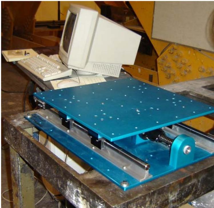
(b.) Photograph of Shake Table and Operation PC (Data Acquisition not shown)
