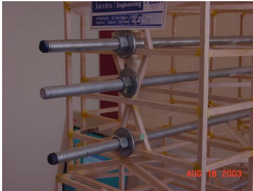
(a.) Example of insufficient support for threaded bars preventing the requisite tightening of the nuts, thereby permitting the bars to slide with respect to the structure during shaking. (The photo was taken at the 2003 competition, when weight distribution differed from this year's configuration.)
