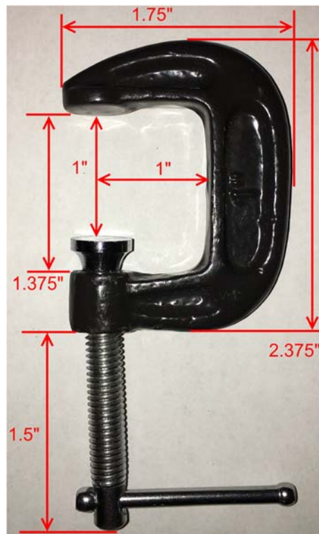
Dimensions of c-clamps used to secure roof accelerometer.
