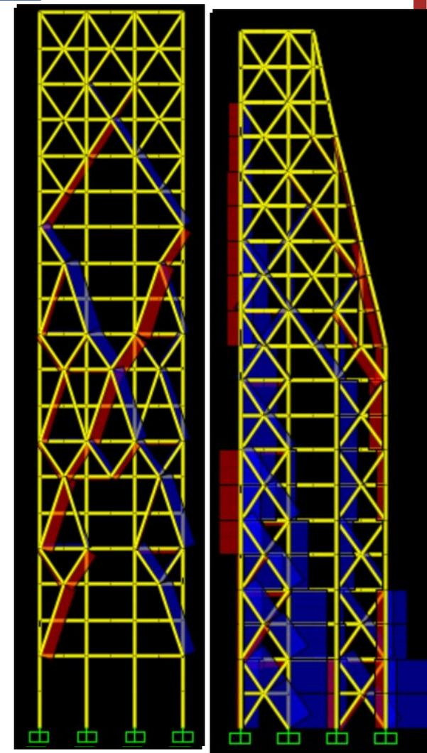
Figure 10.a. Internal Axial Forces for Retrofitted Structure, East Elevation View
