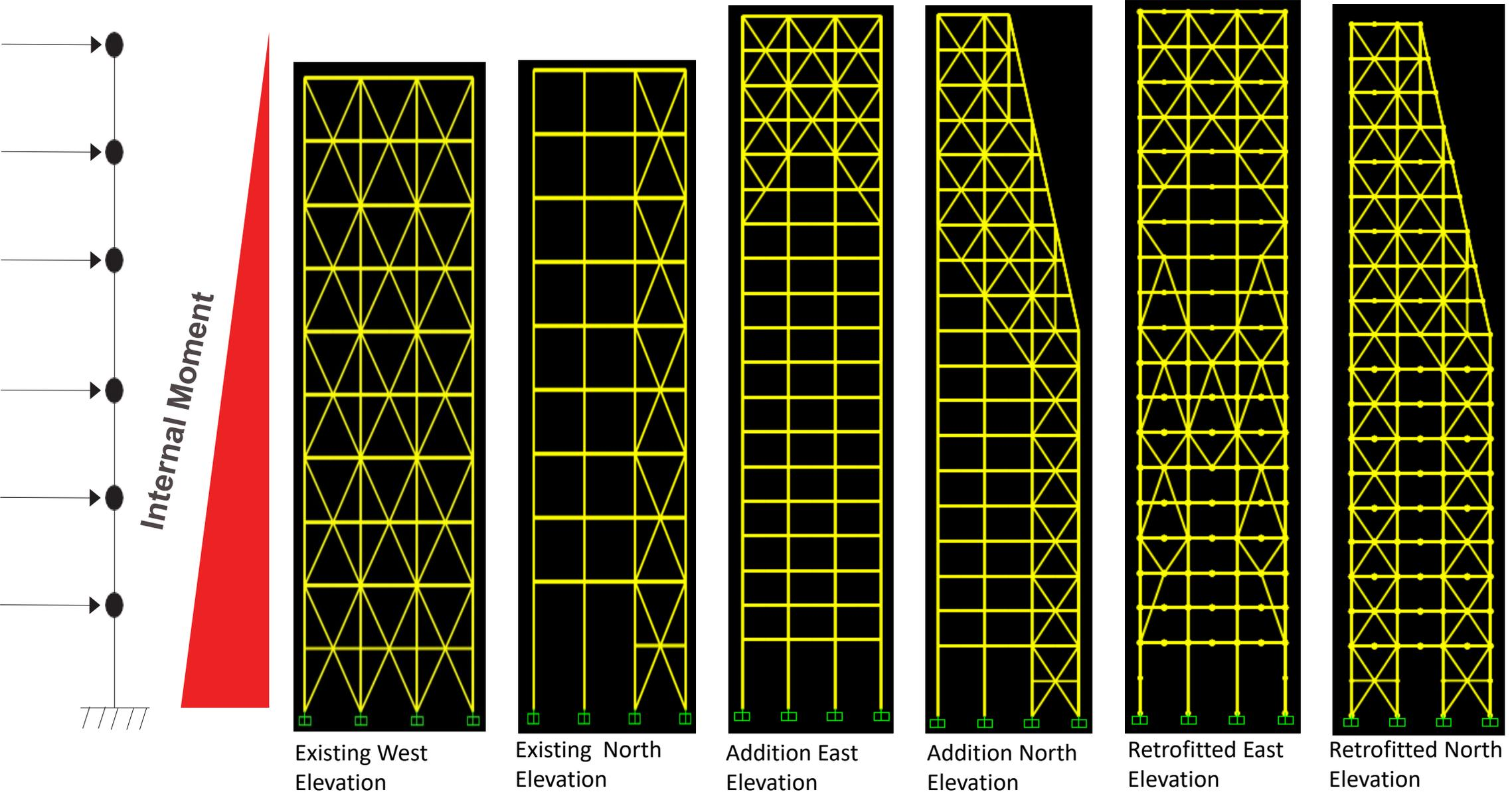
The structure was analyzed using the Time History data provided by the SLC. Uniform loads were applied to the structure to the certain beams using tributary width. Self weight of the structure was also included in the analysis. The results retrieved from the SAP 2000 analysis are shown below. The results after the retrofitting were significantly better than the results of the existing and existing with out the retrofit.
