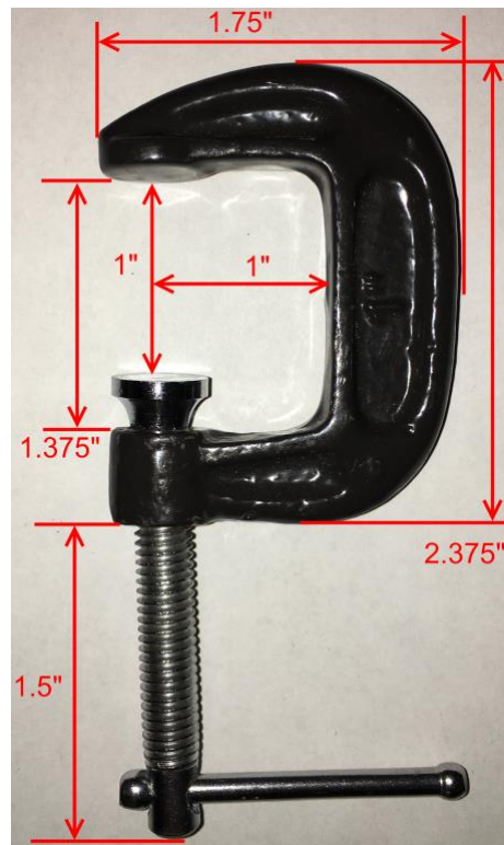
Figure 20: Location of roof accelerometer and dimensions of c-clamps used to secure roof accelerometer (1" = 2.54 cm).
