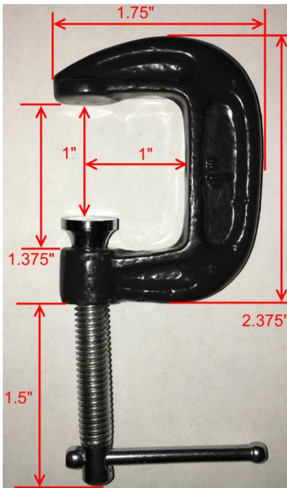
Figure 18 Location of roof accelerometer and dimensions of c-clamps used to secure roof accelerometer (1" = 2.54 cm).
