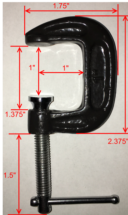
Figure 18 Location of roof accelerometer and dimensions of c-clamps used to secure roof accelerometer (1" = 2.54 cm).
